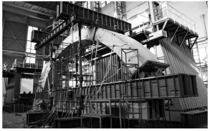
The complex is dedicated for static and cyclic tests. The tests are conducted on strength test stands, reinforced floor and wall.
